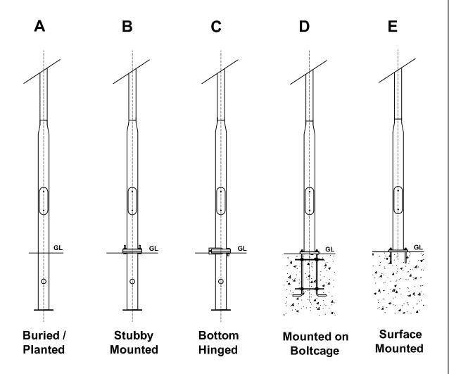
Options A, B & C are Buried / Planted by means of compacted soil (these options can also be secured with concrete, but not essential)
